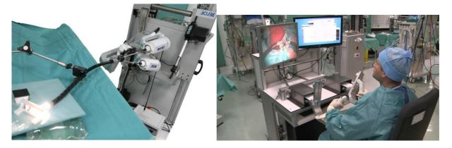
Fig. 1. left: Slave part of the STRAS platform. Right: Telemanipulation during in vivo trials.
